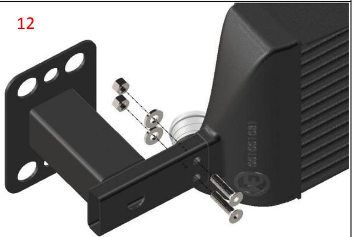
*Attach the WT crossbars to the WT intercooler. Use the supplied M8 allen screws, washers and nuts (as you can see in picture 12). Make sure the crossbar with the welded nut on its inside is placed on the passenger side.*
