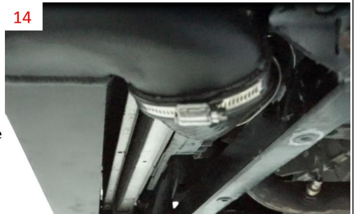
*Attach the WT silicone hoses to the WT intercooler. For this purpose use the supplied hose clamps (13 - 14).*
