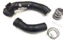
N55 charge pipe with Clip and Oring
